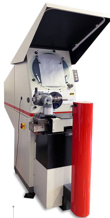
The microscope profile projector for the verification of the most imperceptible of imperfections is the most recent addition to the continuous evolution of Montenero.
